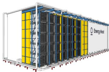
Figure 14 A unit of concrete tubes for thermal energy storage and a container unit filled with concrete tubes for the storage of thermal energy (Energy-Nest, 2020).
