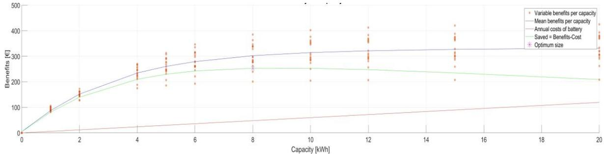
**Figure 2: Savings and costs related to different battery sizes**
