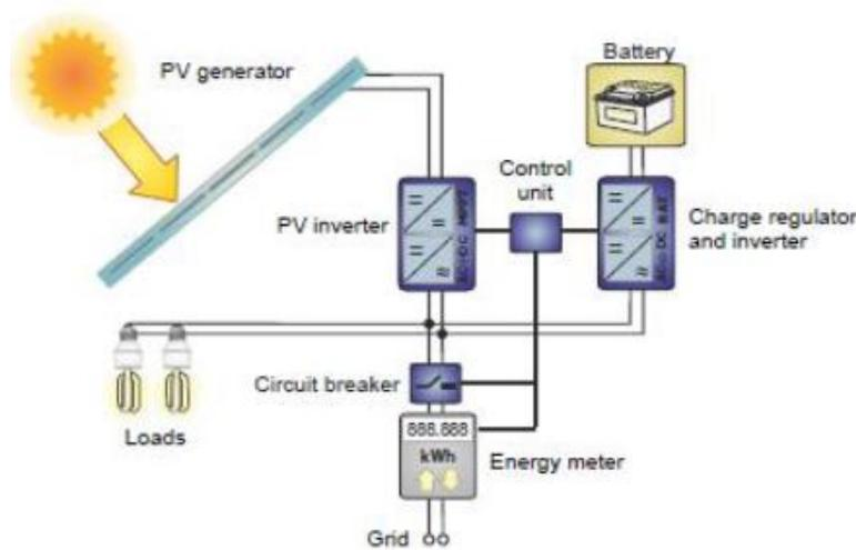
**Figure 1. Schematic of energy system of NZEB**
