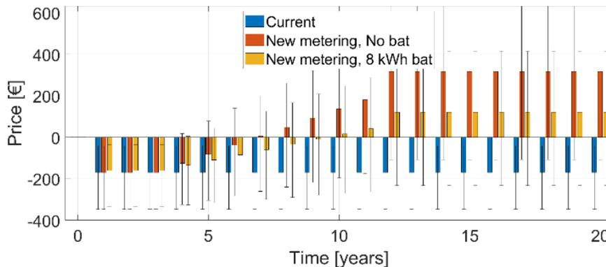
**Figure 3: Energy price current metering agreement compared to new metering agreement**
