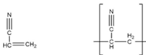
Figure 3.19: Chemical structure of acrylonitril (left structure), main monomer of the polymer polyacryl (right structure).
