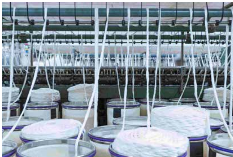
Figure 2.4: Cotton sliver production, a step in the yarn spinning process.
