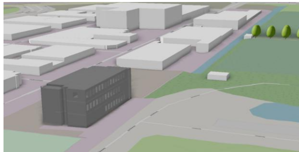
Fig. 3. ArcGIS visualization of Donor Building BIM model (gray) on OSM with World Elevation 3D.
