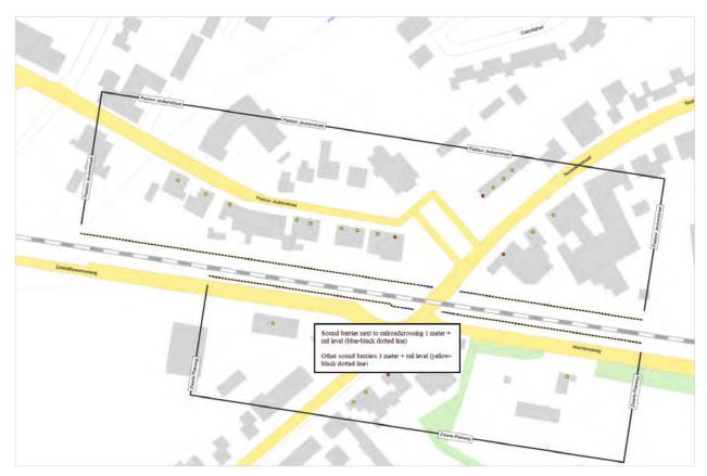
BS = Rail top: the height of the sound barriers is always measured from the top of the rails; this measurement does not depend on the local situation.
